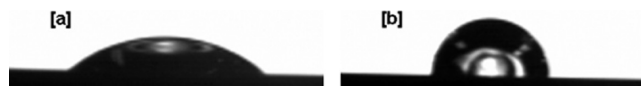
FIGURE 5. Water contact-angle measurements done on (a) pristine AF45 glass and (b) carbon-coated AF45 glass made using PR (10:1) as the precursor ( \sim 5 nm thick).
